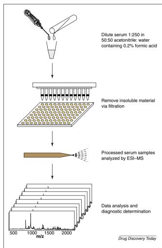
Figure 3. Sample-processing method used to analyze serum samples using the OvaCheck™ diagnostic platform. In this method, raw serum is diluted and filtered to remove particulates. The proteomic pattern of the filtered samples are then acquired using electrospray ionization mass spectrometry. As with SELDI-TOF–MS analysis, bioinformatics is used to discover peaks that enable the source of the serum sample (i.e. a healthy or cancer-affected patient) to be determined.
